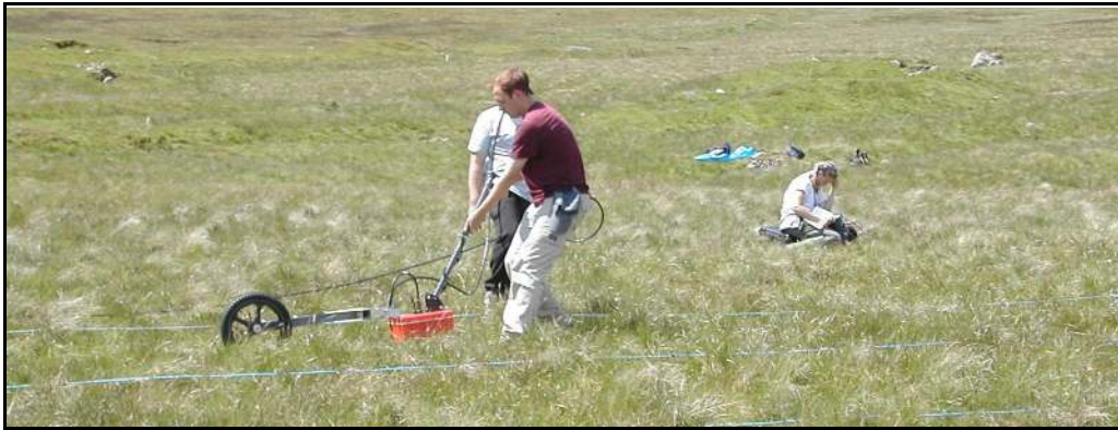
Figure 2 SIR3000 GPR with 400 MHz antenna and survey wheel.
