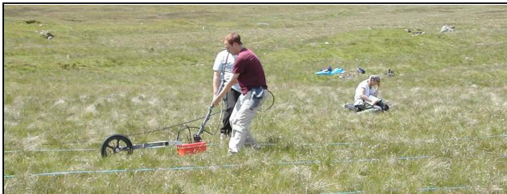
Figure 1 SIR3000 GPR with 400 MHz antenna and survey wheel.
